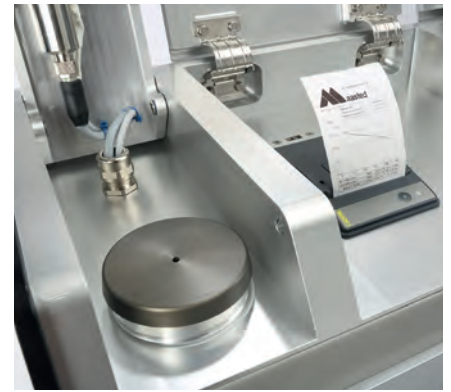
The sample reactor within the ChocoAnalyzer instrument.
